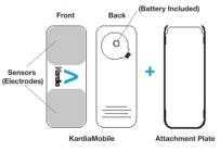
If you choose to attach KardiaMobile Hardware to the phone, adhere the optional attachment plate to the back of the phone.
